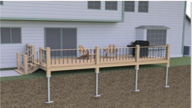
Cross-Section example showing helical pile foundation
